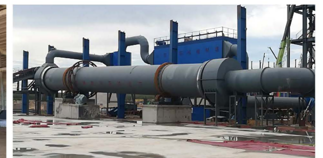
\Phi 2.8 \times 28 m Rotary Drum Drying System
