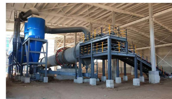
\Phi 2.6 \times 24 m Rotary Drum Drying System
