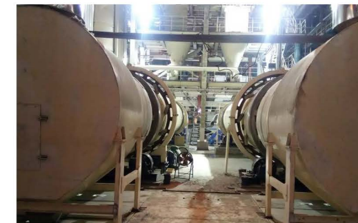
\Phi 2.4 \times 18 m Rotary Drum Drying System
